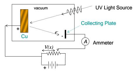
The energy of the emitted electrons (from the Copper plate) is a function of the frequency of light from the light source. The photoelectric experiment can be used to measure Planck's constant directly.
